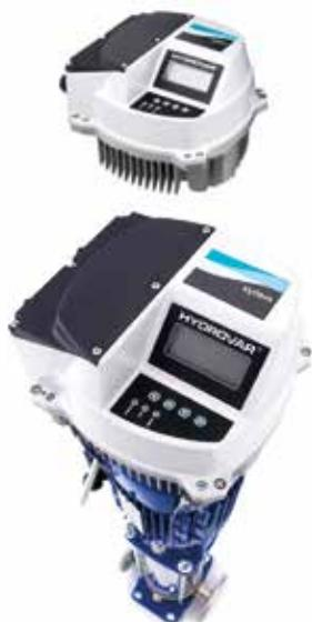
Hydrovar units installed on to a fixed speed booster set not only eliminates the need for a control panel but also introduces a soft start function, that when combined with the benefits of running a pump at a variable speed, can prolong the life of the pump and the water system. By reducing the in-rush current when the pump is turned on, parts such as motor bearings and pipe fittings are protected from hydraulic shock than can cause cavitation and breakdown.
