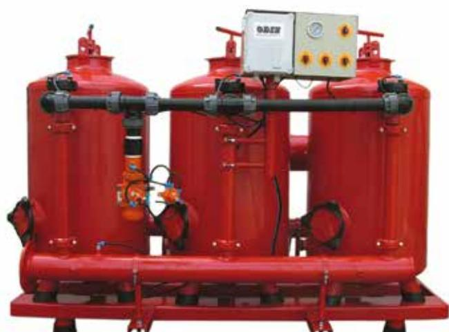
TYPE C MOBILE ARRAYS come complete with sand filters, a screen filter as a back-up and control filter, flushing valves and electronic controller. They come completely assembled and mounted on a steel pallet which can be moved to different locations.
