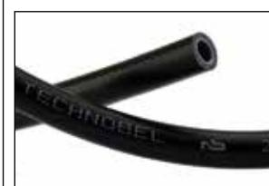
A hose suitable for agrochemicals and compressed air in arduous industrial conditions. A four layer thermoplastic design with braided reinforcement and a thermopolymer lining give extra resistance for a longer life.
