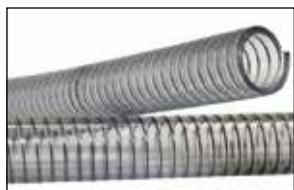
A transparent, flexible suction/ delivery hose with a galvanised steel spiral making it highly resistant to vacuum and crushing. Smooth inner walls give low flow losses and make this hose easy to clean. Food quality hose suitable for temperatures up to 40°C.
