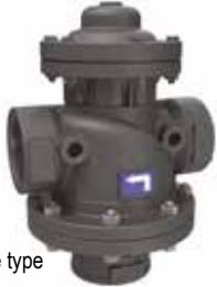
The BERMAD Model IR-2x2-350-P is a compact 3-port valve, in a T configuration. It is double chambered, hydraulically operated, and diaphragm actuated. Designed for automatic backwashing of filtration systems.
